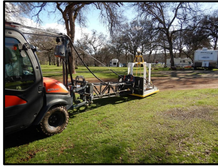
Left: Advanced metal detector equipment being pulled over flat terrain.
