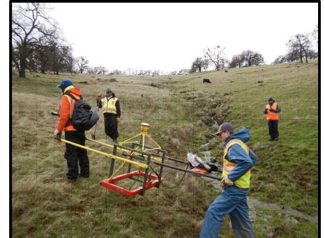
Left: Advanced metal detector equipment being pulled over flat terrain.
